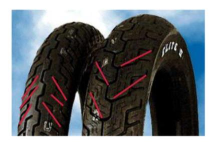
However, if you look at the front tire tread pattern of the new Dunlop Elite II's (K491) they are aligned in exactly the opposite way. That is, they tend to channel water towards the center of the tire. This CANNOT be the most effective way to diminish the odds of hydroplaning! Either the K177 or the K491 is safer on wet streets based on those tread patterns. (I believe that most new street bikes (other than Honda) come with tires treaded like the K491's.)
