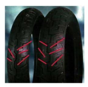
If you look at the tire tread pattern you will also see that the grooves are cut in such a way as to tend to channel water away from the center of the tire if it is rotating in accord with the arrow stamped on the side of the tire. This seems to be consistent with what the Dunlop factory rep advised in his latest message to me on the subject.
